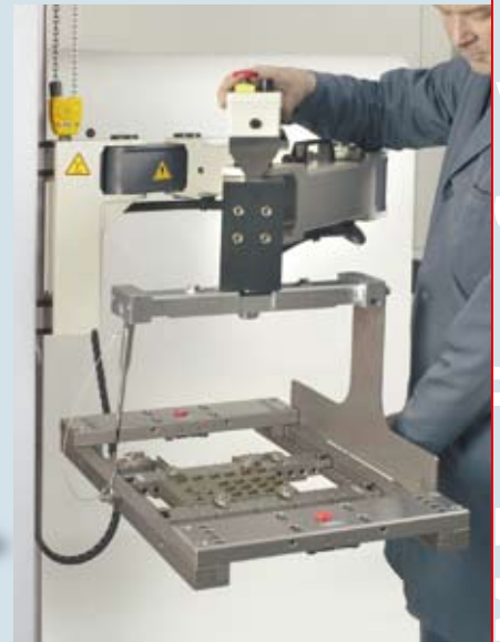
With the EROWA Lift, you can load/unload the clamping frames onto/from the machine quickly and safely.
